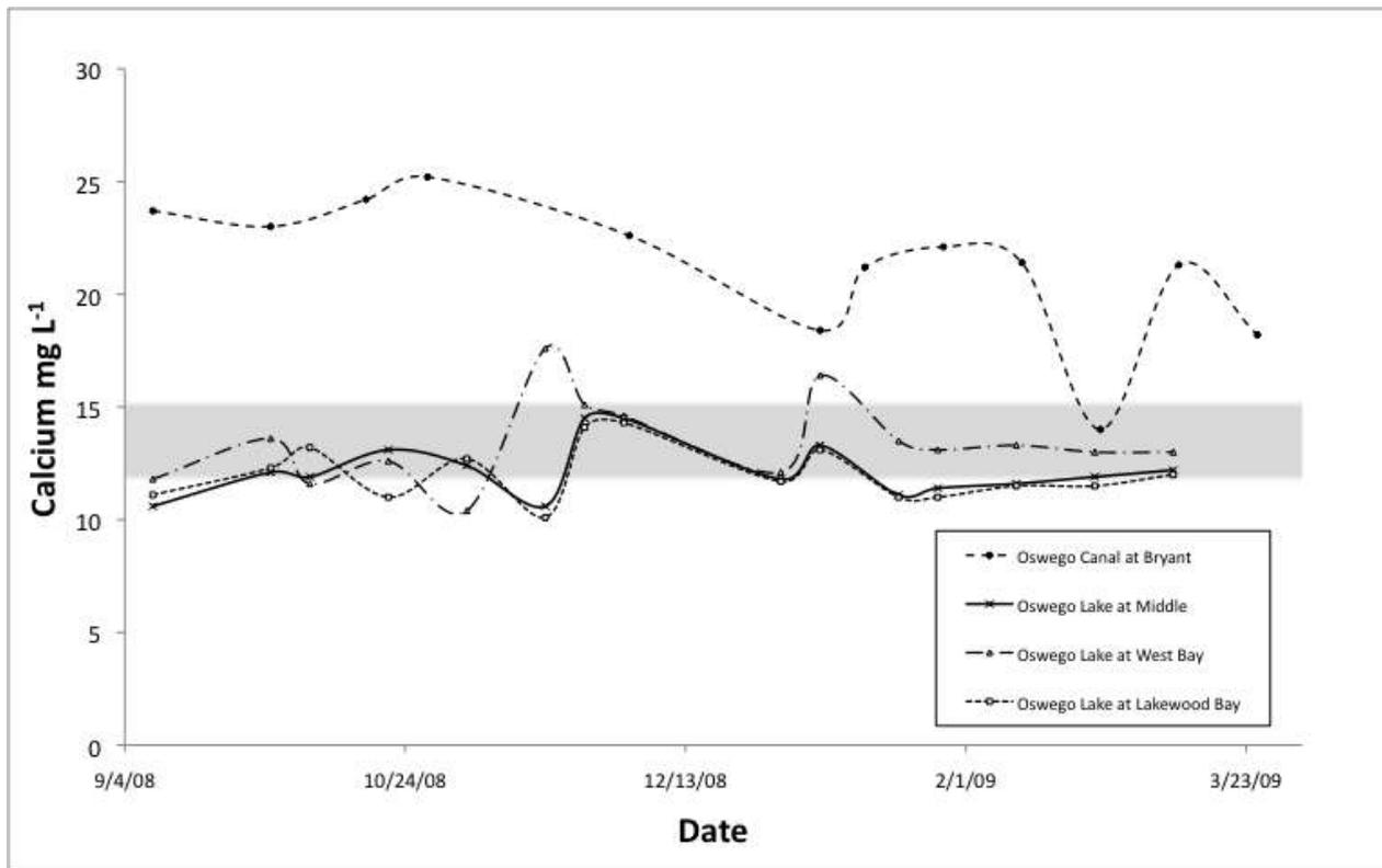
Figure 2. Calcium levels (mg L<sup>-1</sup>) at four regions of Oswego Lake. West Bay and Lakewood Bay samples taken from 1m, middle taken at 5m, Oswego Canal taken at 0.5m. Grey bar indicates average minimum calcium threshold in North America for zebra and quagga mussel survival, though populations have been found at calcium levels below 12 mg L<sup>-1</sup>.
